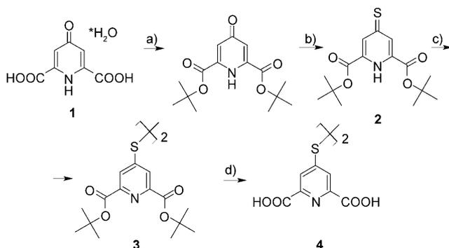
Scheme 2. Synthesis of dimeric 4,4'-dithiobis-dipicolinic acid (**4**): a) isobutylene, HClO<sub>4</sub>, CH<sub>2</sub>Cl<sub>2</sub>; b) Lawesson's reagent, toluene; c) H<sub>2</sub>O<sub>2</sub>, Bu<sub>4</sub>NCl, CH<sub>2</sub>Cl<sub>2</sub>/H<sub>2</sub>O; d) trifluoroacetic acid (TFA), CH<sub>2</sub>Cl<sub>2</sub>.
